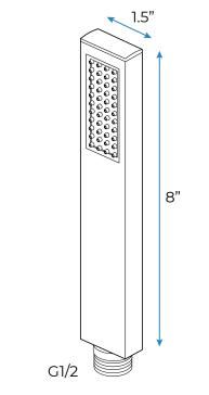
Flow Rate: 2.0 GPM / 7.6 LPM
